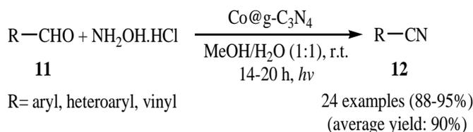
**Scheme 5.** Co@g-C<sub>3</sub>N<sub>4</sub> catalyzed cyanation of aldehydes **11** with NH<sub>2</sub>OH·HCl.
