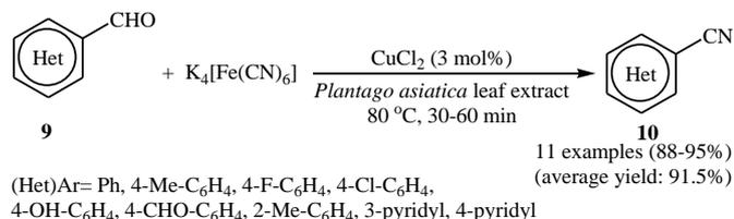
**Scheme 4.** Cu NPs-catalyzed cyanation of aromatic aldehydes **9** with  $K_4[Fe(CN)_6]$ .
