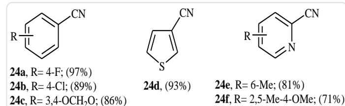
**Scheme 13.** Pt NPs/C-catalyzed ammoxidation of benzylic alcohols **23** with gaseous ammonia developed by Stahl.
