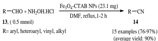
**Scheme 6.** Fe<sub>3</sub>O<sub>4</sub>-CTAB NPs catalyzed synthesis of nitriles **14** from aldehydes **13**.
