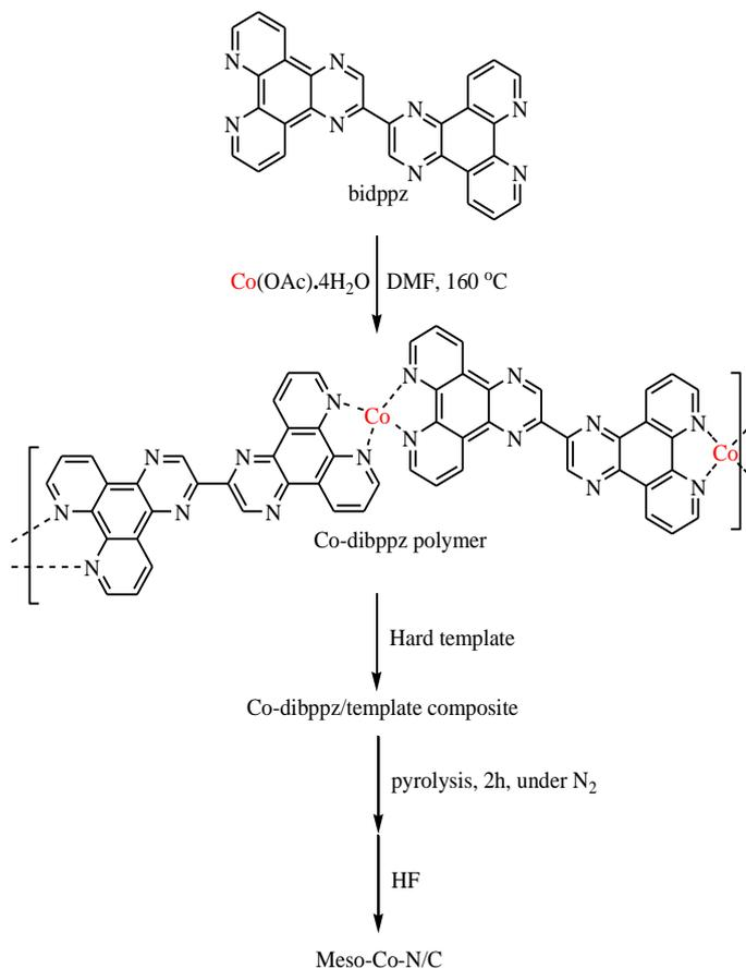
**Fig. 6** Synthetic route for preparation of meso-Co-N/C.
