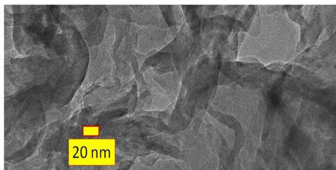
**Fig. 4** TEM image of Co@g-C<sub>3</sub>N<sub>4</sub> photocatalyst.
