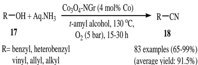
**Scheme 9.** (Co<sub>3</sub>O<sub>4</sub>-NGr/C)-catalyzed aerobic ammoxidation of primary alcohols **17** with ammonia.
