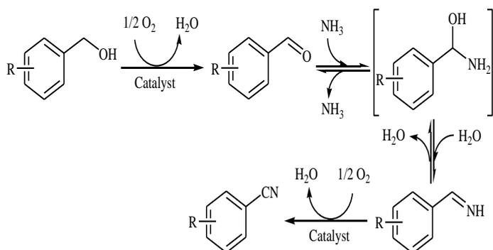
**Scheme 11.** Mechanistic proposal for the reaction in Scheme 10.
