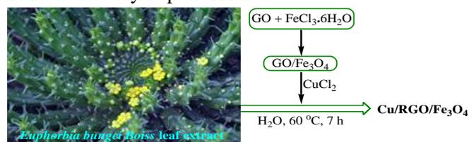
**Fig. 3** Schematic diagram showing the formation of Cu/RGO/ $Fe_3O_4$  NPs.
