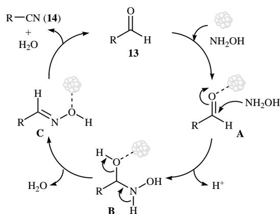
**Scheme 7.** Proposed mechanism for the reaction of aldehydes **13** with NH<sub>2</sub>OH.
