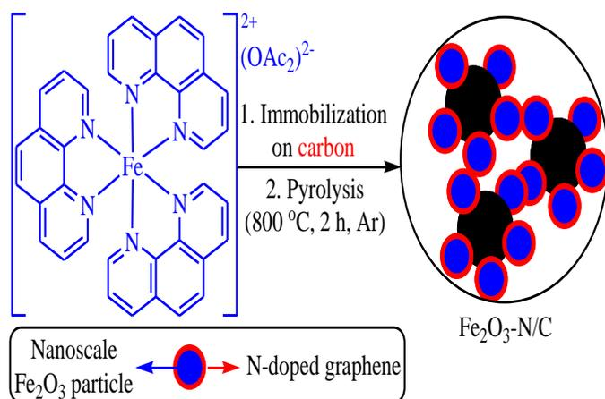
**Fig. 5** Synthesis of nitrogen doped graphene activated nanoscale Fe<sub>2</sub>O<sub>3</sub>-particle supported on carbon (Fe<sub>2</sub>O<sub>3</sub>-N/C).
