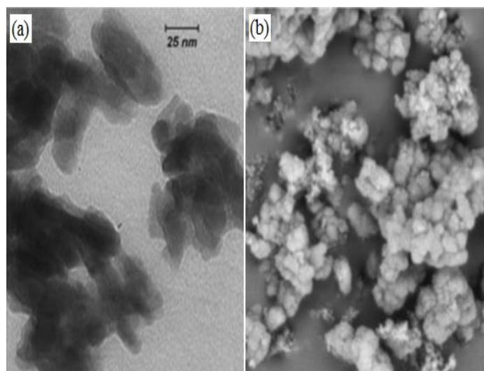
**Fig. 7** (a) TEM images of La(OH)<sub>3</sub>/Fe<sub>3</sub>O<sub>4</sub>, (b) SEM image of La(OH)<sub>3</sub>/Fe<sub>3</sub>O<sub>4</sub>.
