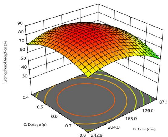
**Fig 4a.** 3D Response surface for interaction between time and dosage for 4-BP adsorption
