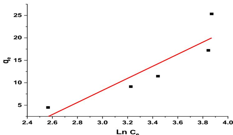
Fig 7. Temkin isotherm plot for 4-BP adsorption on BiFeO<sub>3</sub>
