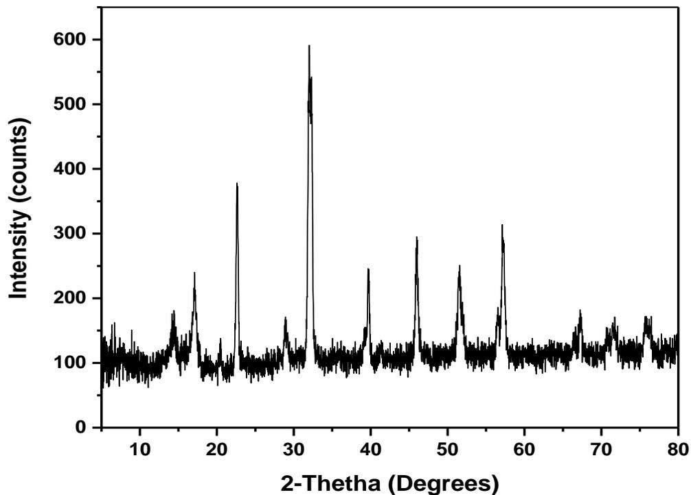
Fig 1. Powder XRD pattern of the prepared BiFeO<sub>3</sub> adsorbent.
