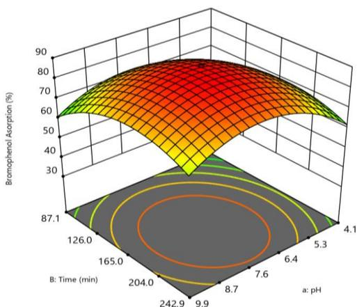
**Fig 4c.** 3D Response surface for interaction between time and pH for 4-BP adsorption
