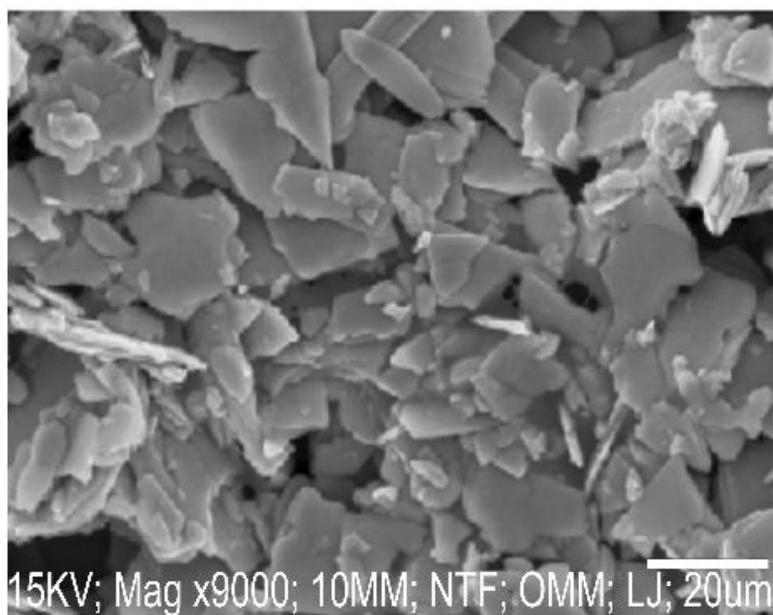
Fig 2b. SEM image of the BiFeO<sub>3</sub> at 20 μm magnification
