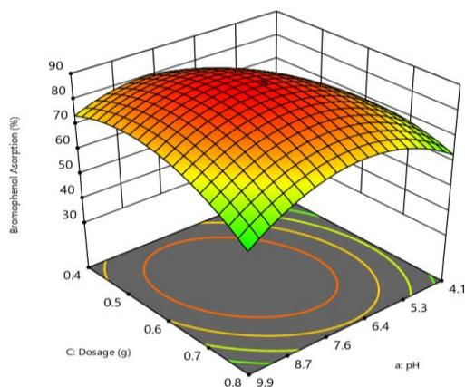
**Fig 4b.** 3D Response surface for interaction between pH and dosage for 4-BP adsorption
