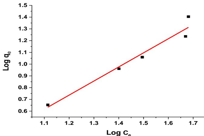
Fig 6. Freundlich isotherm plot for 4-BP adsorption onto  $\text{BiFeO}_3$
