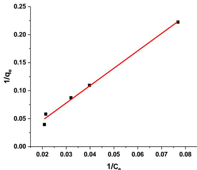
Fig 5. Langmuir isotherm plot for 4-BP adsorption onto  $\text{BiFeO}_3$
