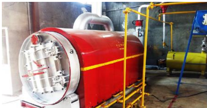
Figure 1. The designed high performance rotary kiln co-pyrolysis system
