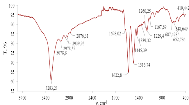
Figure 3. The IR spectrum of “HF” containing silver
