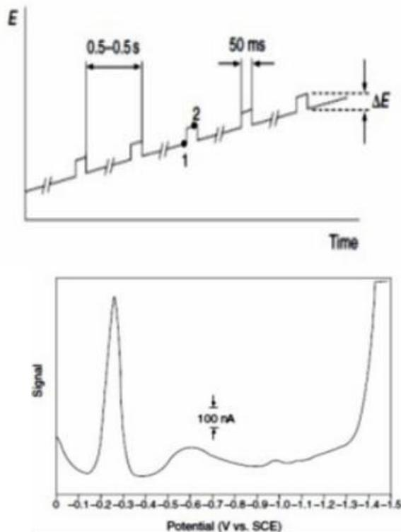
**Fig. 4.** Potential-time and current-potential diagrams in normal pulse voltammetry
