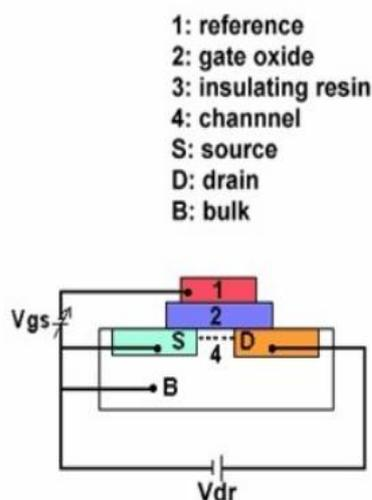
Fig.7. Field-effect transistor
