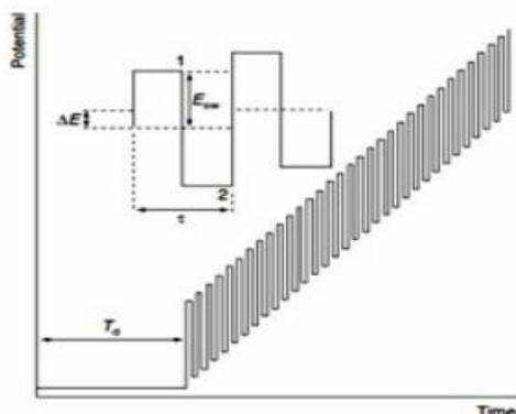
**Fig. 5.** Potential-Time diagram in square wave voltammetry
