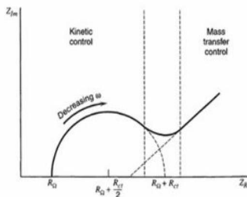
**Fig. 6.** Impedance diagram of electrochemical system
