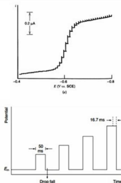
Fig. 3. Potential-time and current-potential diagrams in normal pulse voltammetry
