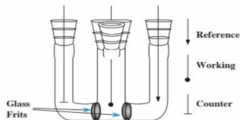
**Fig.1.** Electrochemical cell of three electrodes system
