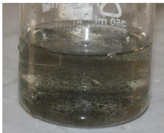
Figure 2 (b): The image of CNTs after activation is dispersed in water and suspended as fine particles.
