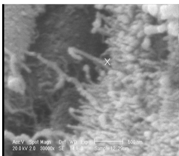
Figure 4 - SEM image after the activation of CNTs and the separation of Nano-tube powder without the use of centrifuge with an x30,000 magnification.
